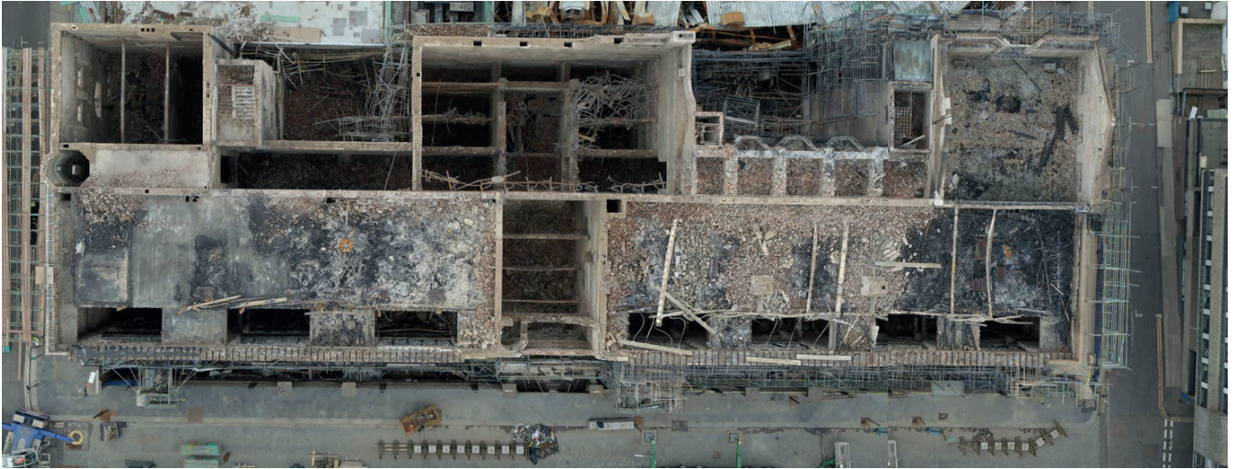
Drone's eye view and digital model of the burnt out shell of Glasgow School of Art following the second fire (Images: Glasgow School of Art)
